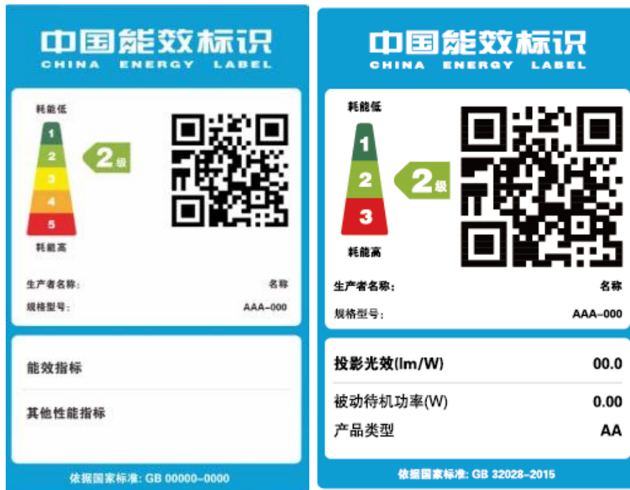
Figure 18: China - Energy label with 5 levels (left) and Energy label with 3 levels (right)
